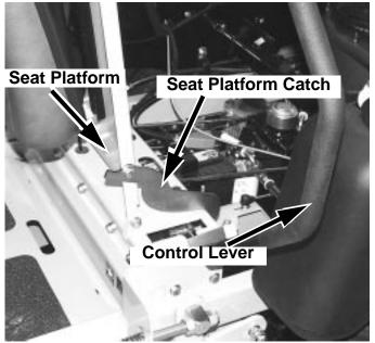
Access to Engine and Hydraulic Pumps 19070
